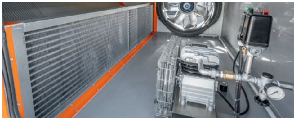
Additional heater battery (optional) and compressor
