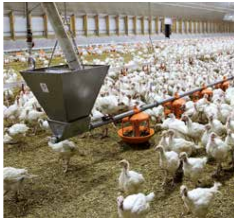
Imperator pan feeder for turkey growing
