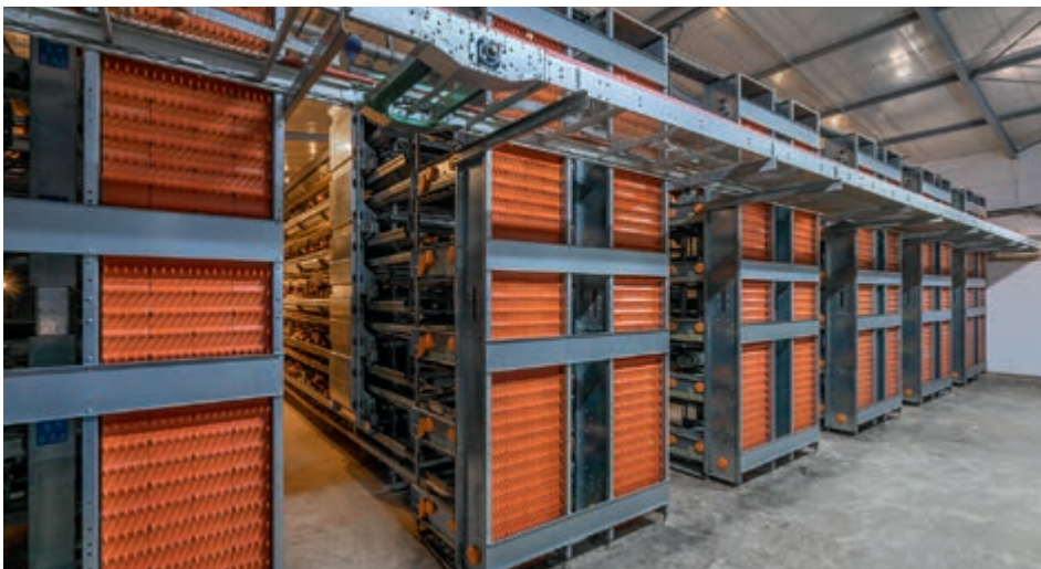
Example of a UV 600 layer system, six tiers with feed cart
