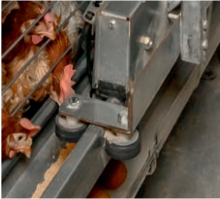
Rubberised rollers with ball bearings ensure quiet and smooth running of the feed cart
