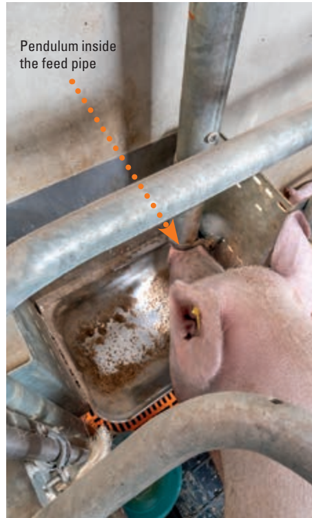
Sensor-controlled: a sow actuating the pendulum inside the feed pipe
