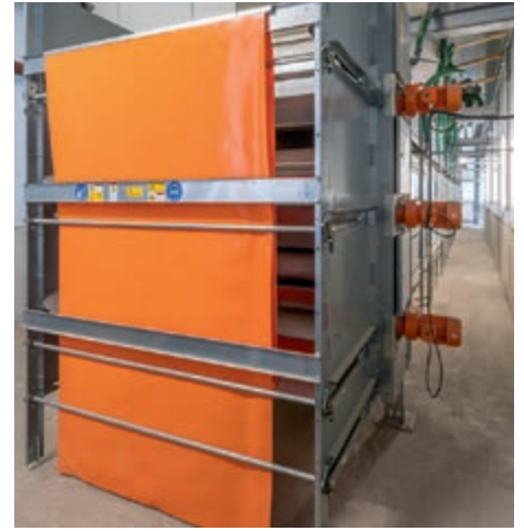
Six-tier manure drying tunnel
