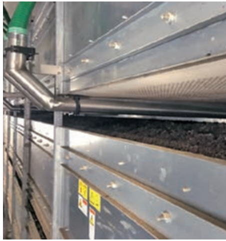
A distribution system sprays the liquid proportion evenly onto the material that is to be dried
